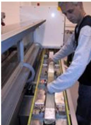
**PART B:** It will be focused in the analysis of sediment cores with the ITRAX- Core Scanner of the University of Vigo. ITRAX is a laboratory instrument developed for measurements of the variation of density and chemical element composition along sediment cores. The instrument analyses flat samples as well as split cores. With the combination of optical imaging, high-resolution
